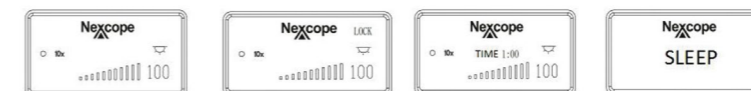
Start & working mode Lock mode Turn off the light after leaving mode standby mode
